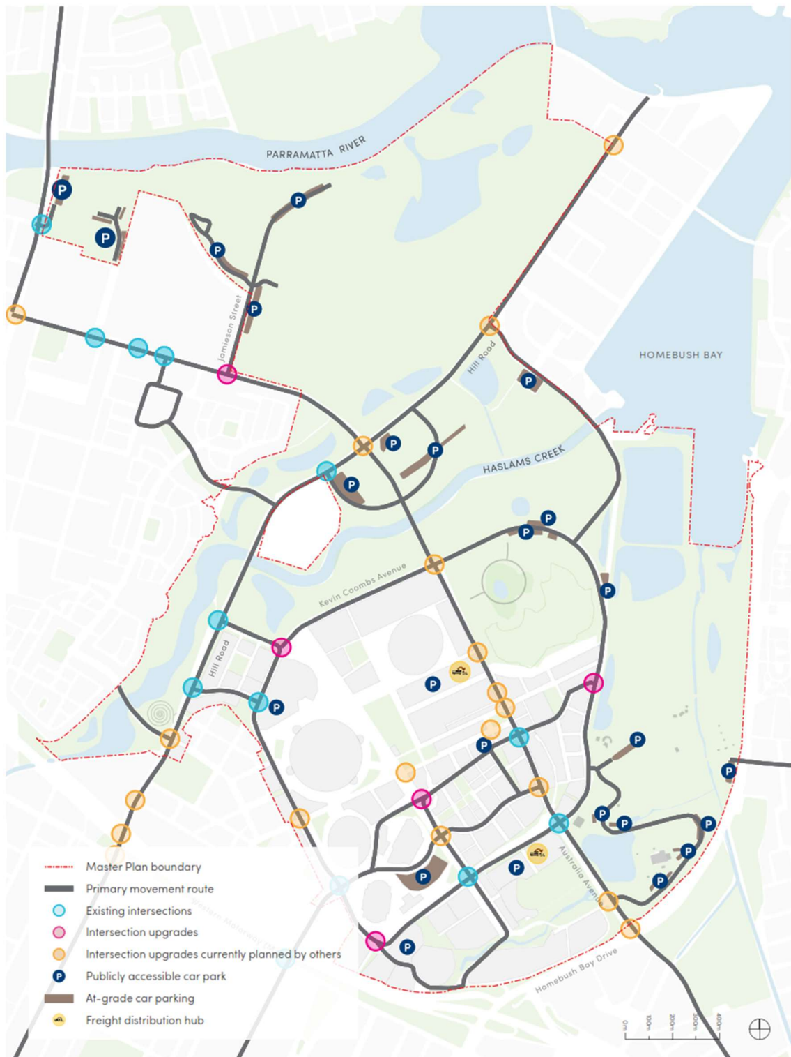
Figure 9: Access routes and intersection upgrades
